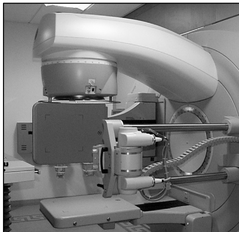
Figure 1: The Synergy system with retractable kV X-ray tube (right) and opposing kV imaging panel.
